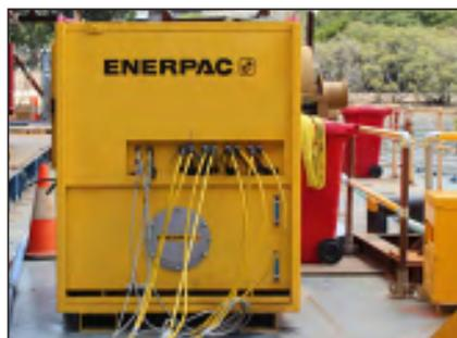
▼ A SyncHoist system used to align steel blocks of the ship's control tower sections allowing gradual lifting and positioning of the load.
