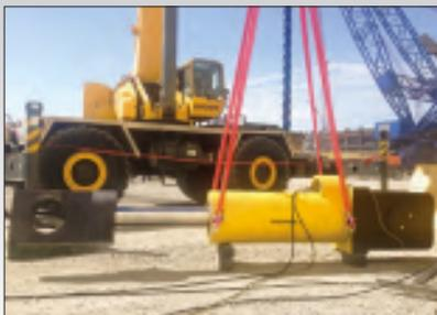
◀ One of three custom SyncHoist cylinders used to place a 1,140-ton nuclear plant module.
