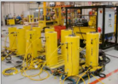
◀ Custom cylinders with embedded sensors for bridge construction.
