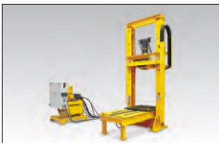
◀ *100-Ton Press for Assembly of Spring-Loaded Cylinders*
